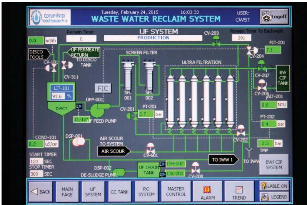
The waste water reclamation system helps to reduce the consumption of potable water.
